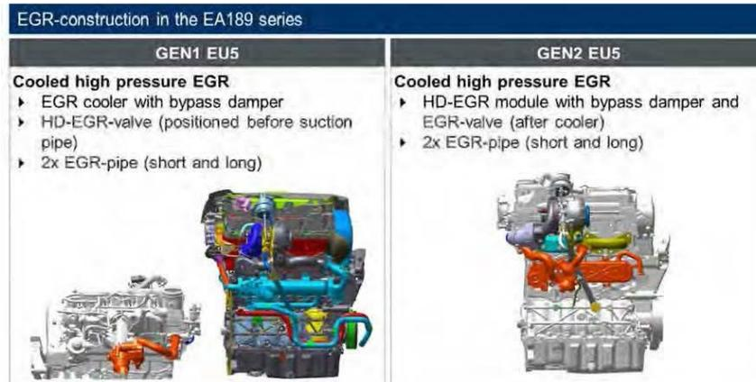
24. The EGR cooler reduces the temperature of the recirculated gas with the use of a heat exchanger.
